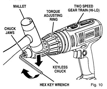
Open the chuck jaws and remove hex key wrench. Remove the chuck screw by turning it in a clockwise direction. See Figure 11.
